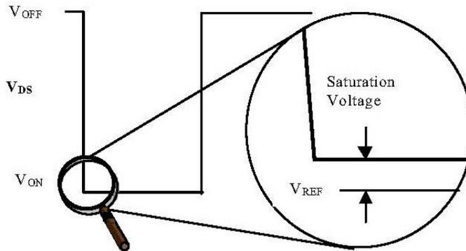
*Figure 3, Saturation Voltage*
