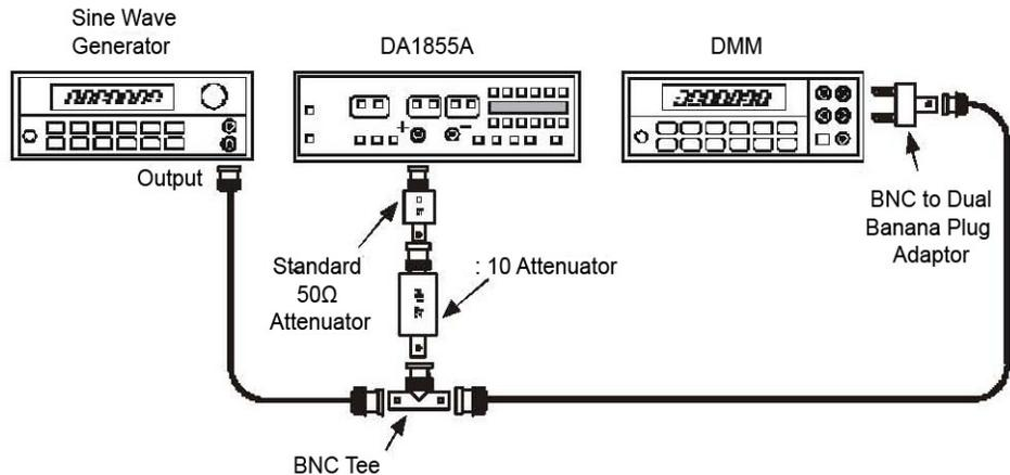
Figure 12, X10 Gain Accuracy Test Setup 3.
