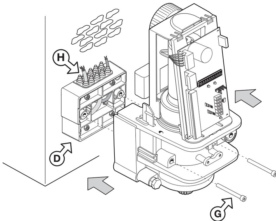
INSERIMENTO FINECORSA MECCANICI - INSERTING THE MECHANICAL TRAVEL LIMITS - MISE EN PLACE FINS DE COURSE MECANQUES
