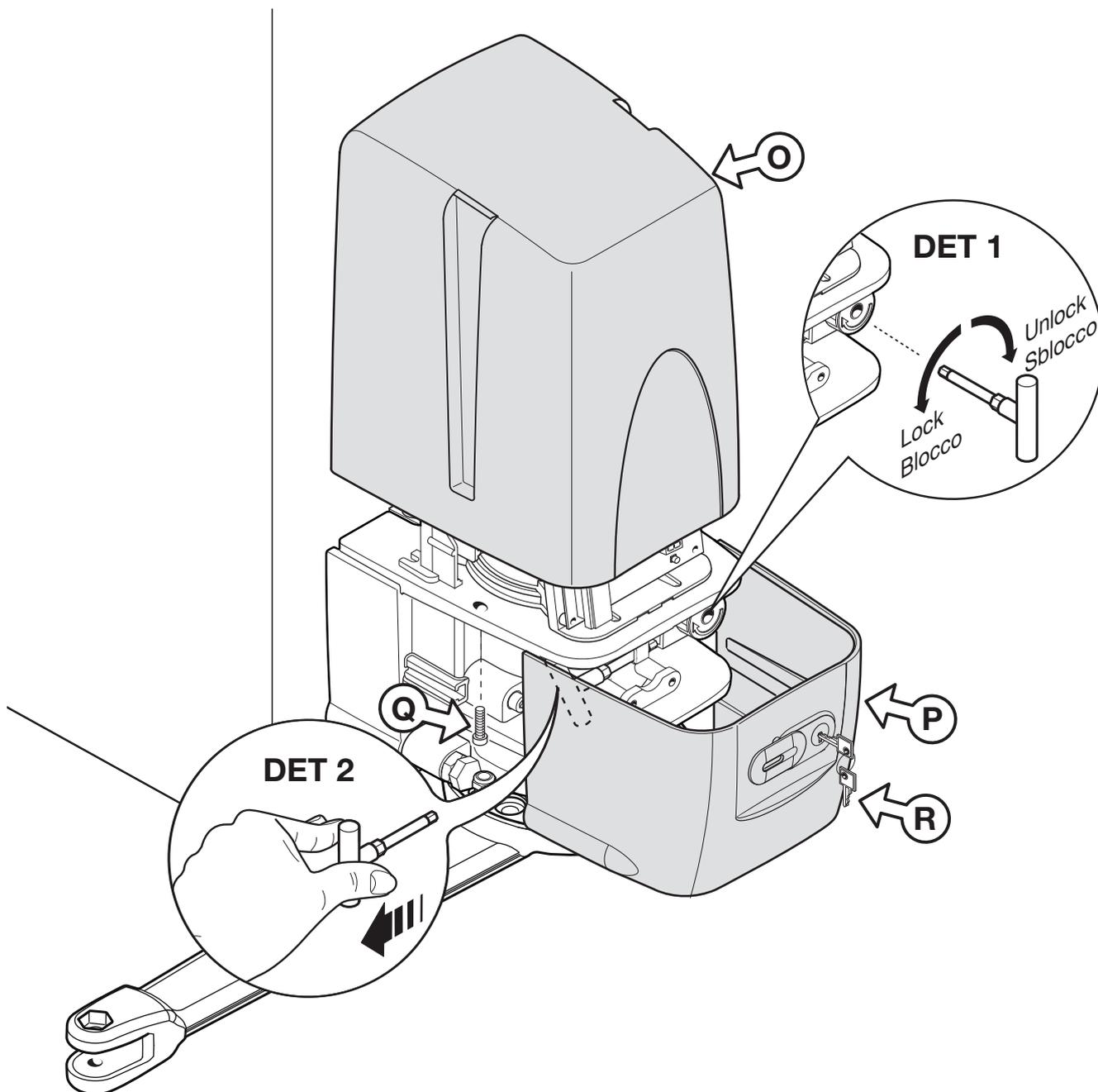
ELETTROSERRATURA (OPZIONALE) - ELECTRIC LOCKING DEVICE (OPTIONAL) - SERRURE ÉLECTRIQUE (EN OPTION)
