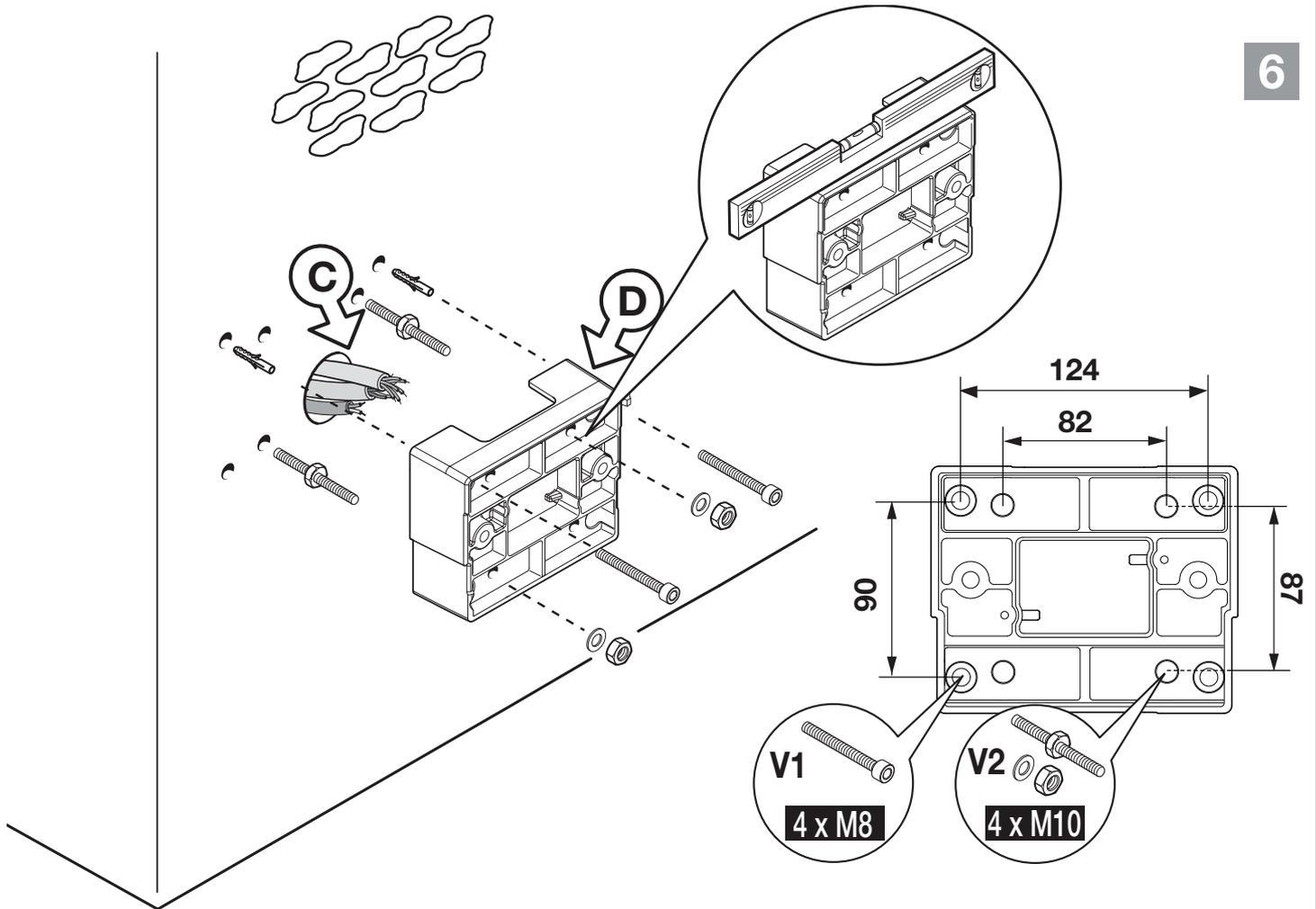
FISSAGGIO PRESSACAVO E PASSAGGIO CAVI - FASTENING THE CABLE CLAMPS AND PASSING THE CABLES
