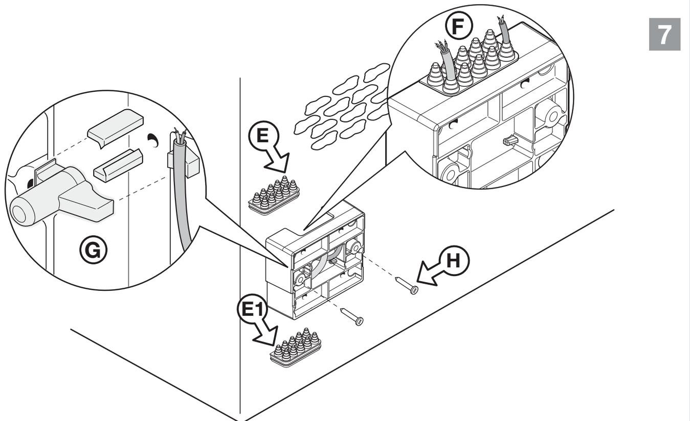
FISSAGGIO MOTORIDUTTORE ALLA BASE - FITTING THE MOTOR TO THE BASE
