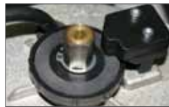
Mechanical twin-disc clutch
