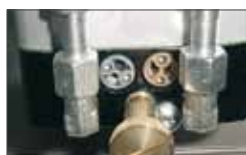
By pass valves for the force adjustment
