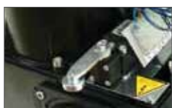
Mechanical limit switch with lever
